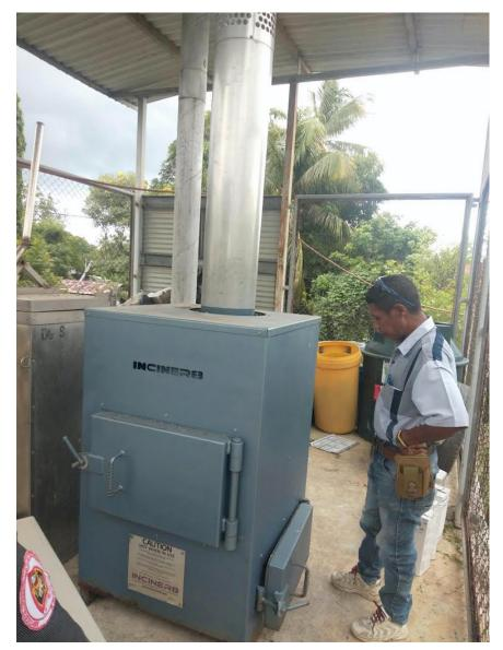
Figure 4-1 - Inciner8 incinerator at Suai Hospital (note: medical waste incinerator to the left not commissioned)
