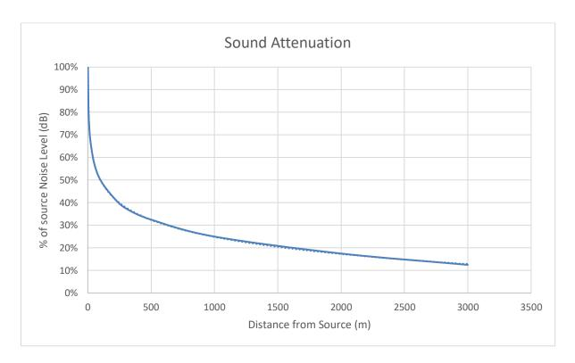
Figure 1-1 - Attenuation Rate of Sound Level in Air
