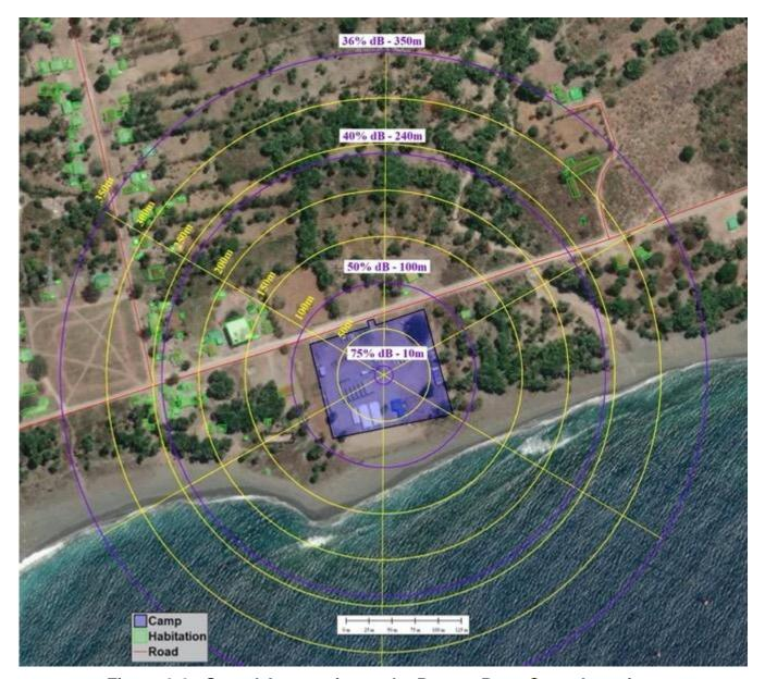
Figure 2-2 - Sound Attenuation at the Betano Base Camp Location
